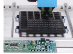
Up&down 2 vision cameras; IC tray; Motor closed-loop control
